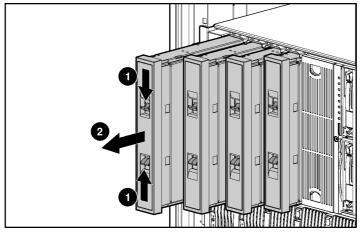
Figure 1-27: Removing a server blade blank
